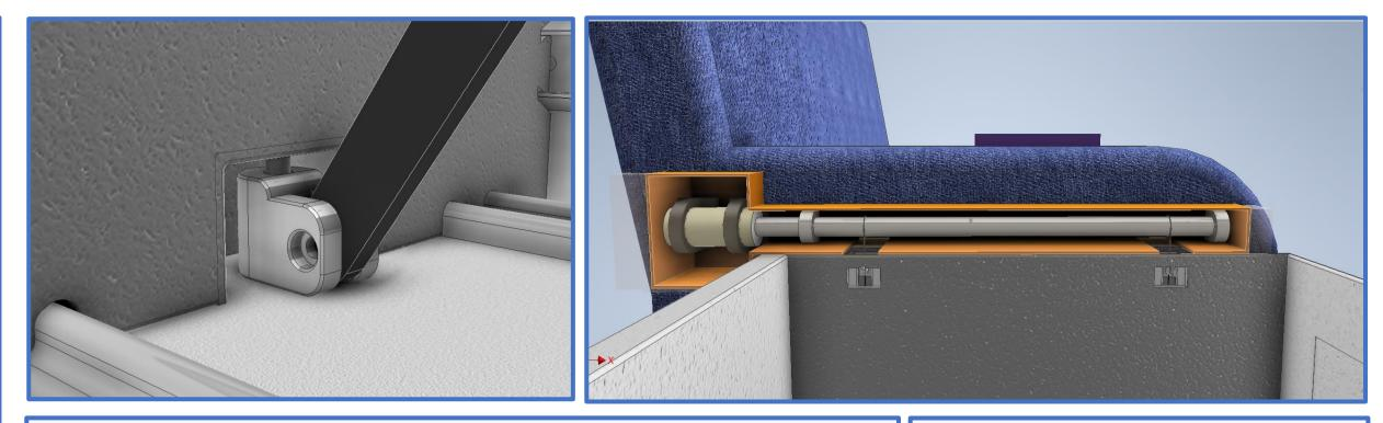
Interlocking pushing component: Connecting slider arm to pin (in the cut-in in the back of Side view of box in **lifted position** with pulley the box). It is fixed to the slider arm with a screw (not shown here) and is connected to cover removed to show motor and pulley the box through only the pin in the hole so that the box can be lifted off it in step 3. system (shaft, bearings, and pulley wire).
