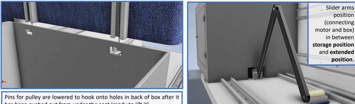
Sensors on the box to halt the mechanism if an obstruction is detected stop its movement. Safety
